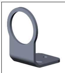
Figure 5: Mounting bracket, adjustable in two axes [ACCTLAB]
