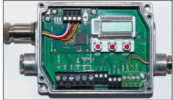
Installation of the Network Interface board into Optris CT Electronic Box
