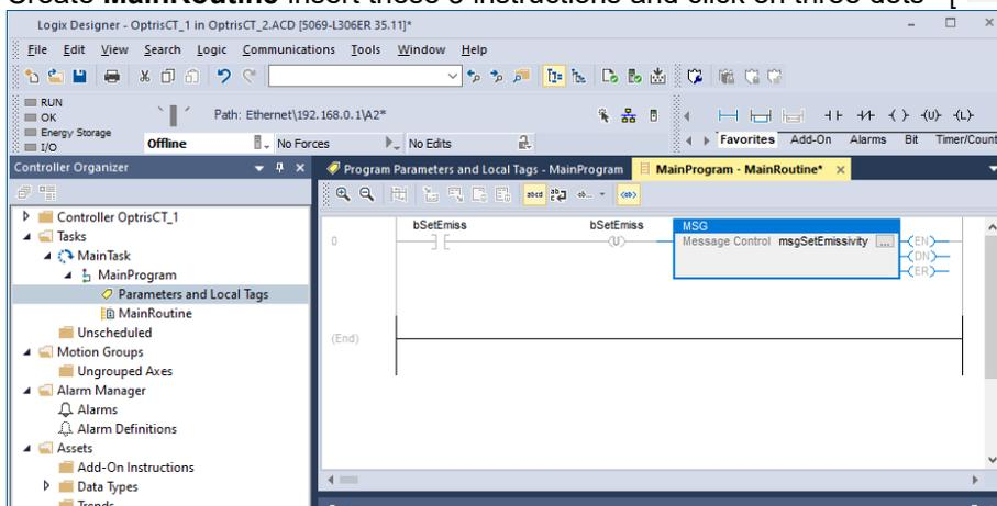
Set the configuration values according to **Table 3**, set the communication path to OptrisCT, and click on **OK**. Download the project to the PLC and start the PLC program in **Run Mode**.
