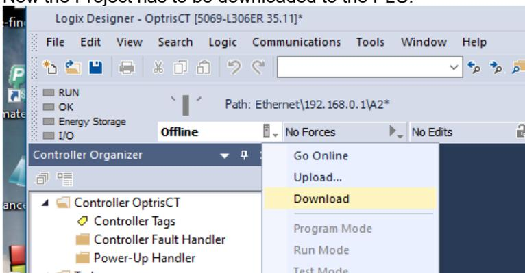
Start the PLC program by clicking **Run Mode**. To see the current cyclic values double-click on the **Controller Tags**.
