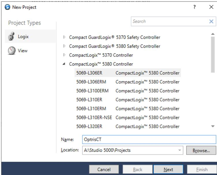
Connect the OptrisCT to the AB PLC port click with the right mouse button on your port in the project and add a New Module.
