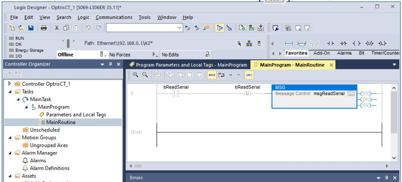
Set the configuration values according to **Table 3**, set the communication path to OptrisCT, and click on **OK**. Download the project to the PLC and start the PLC program in **Run Mode**.
