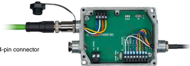
Installation of the Network Interface board
